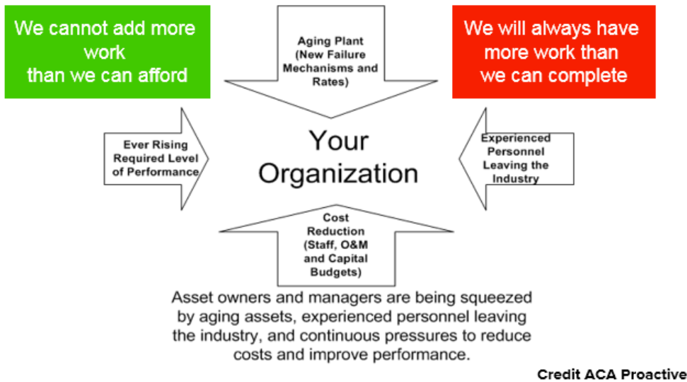
Figure 5 - Drivers for Reliability Centered Maintenance
