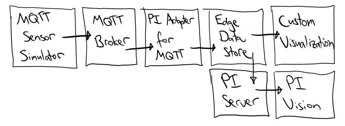
We could have used EdgeCmd to configure EDS, and the commands would have been very similar to the commands we used to configure the adapter. In essence, this architecture uses EDS as a buffer between our Adapter and the rest of our PI System. In a real-word situation, we would make a choice depending on the overall architecture of our system. Seeing as though this class focused on adapters, we did things on the adapter side, but it's possible to do it on the EDS side too.
