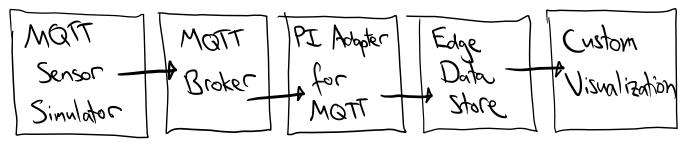
Here's we're pretending our training environment VM is out in the field – "on the edge" – and we'd like to collect data from an MQTT broker and store it locally in an Edge Data Store, for access by custom visualization software running locally on our device. If you're not familiar with Edge Data Store, you can read the documentation *here*. The PI Adapter for MQTT is bound to port 6010 on our class VM.
