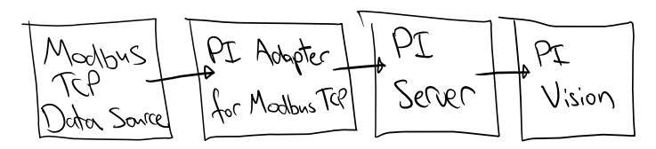
We are going to do this by using the EdgeCmd configuration utility to pass a JSON configuration file to a pre-installed PI Adapter for Modbus TCP.
